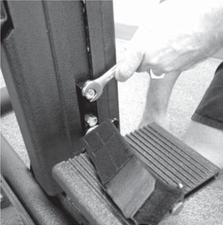
Securely **TIGHTEN** foot pedals with 9/16” wrench.
