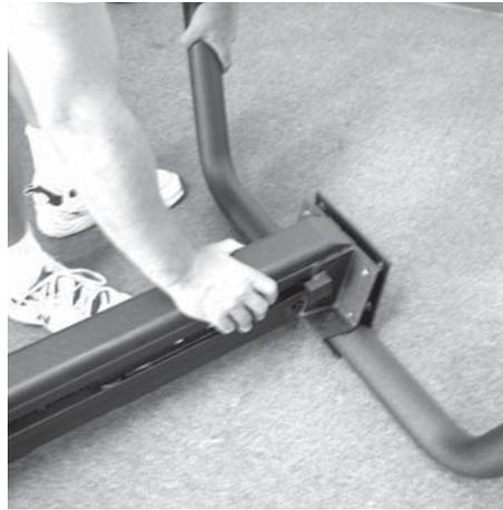
Attach the front curved tubular floor brace to the post. Using four hex head bolts, 3/8" x 5/8" long, screw down until firmly tight.
