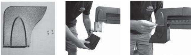
With the post supported or after VersaClimber is upright, slip pump cover into place. Attach with four Phillips pan head screws 1/4" x 3/8" long. **DO NOT OVER TIGHTEN.**
