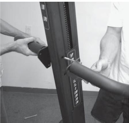
Attach side handrails with (3) hex head bolts 4 1/4” long and (3) 3/8” lock nuts.
